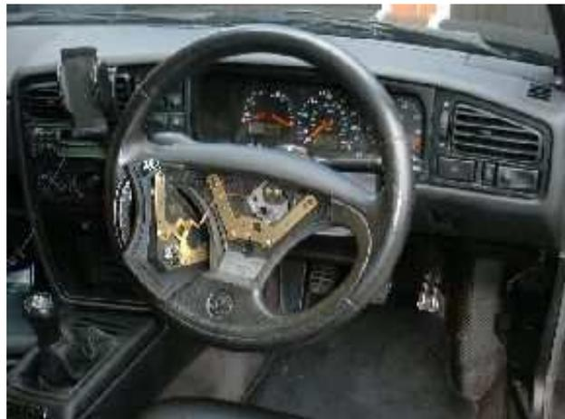
Note the orientation of the steering wheel so you can ensure you put the new one on the same way as the old. I cannot emphasise this enough. It is extremely important if you wish your new steering wheel to look straight when you are driving straight!
